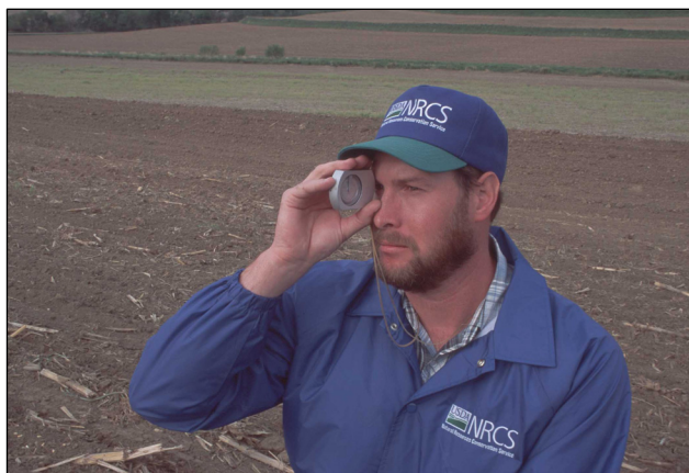
An NRCS conservationist measures slope to determine erosion. Technical assistance is available from NRCS to help plan low cost erosion control systems with farmers.
