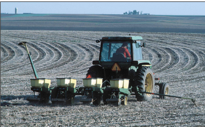
No till planting reduces erosion by keeping more residue on the soil and less soil disturbance.
