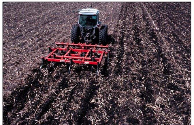
Chisel and other forms of mulch tillage leave more crop residue on the soil surface to protect the soil from erosion.
